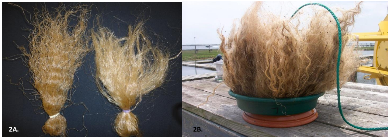
Figure 2A & B. Polyethylene rope strands unraveled into tufts (A) that are inserted in plastic bowl and clay bottom (B) to make a full eel collector.
